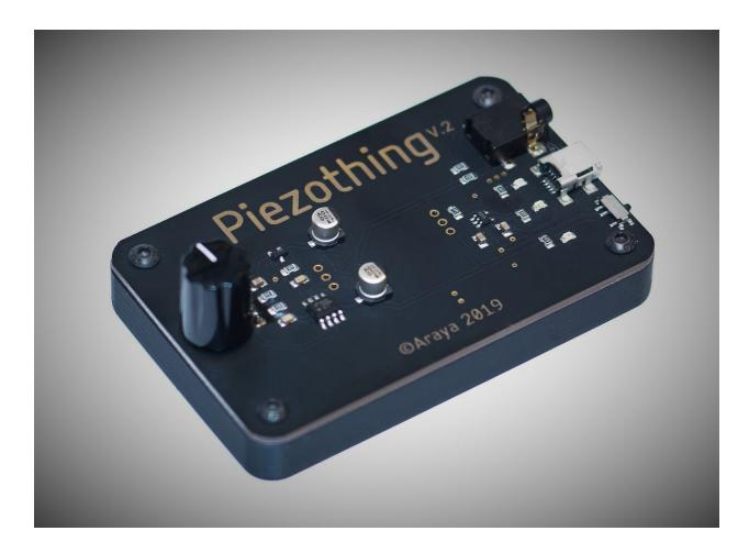
The **Piezothing** is a small feedback instrument containing a piezo microphone, a FET preamp, an amplifier and a small high quality transducer. The mechanical feedback through an object touching the mic and transducer produces both a physical signal vibrating the surface it is placed on as well as an electronic signal available at the headphone/line output.
