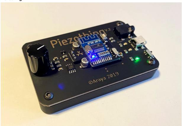
The BT is a Piezothing with an added Bluetooth transmitter board that allows you to stream the audio from the unit to a portable speaker, audio receiver or computer.
